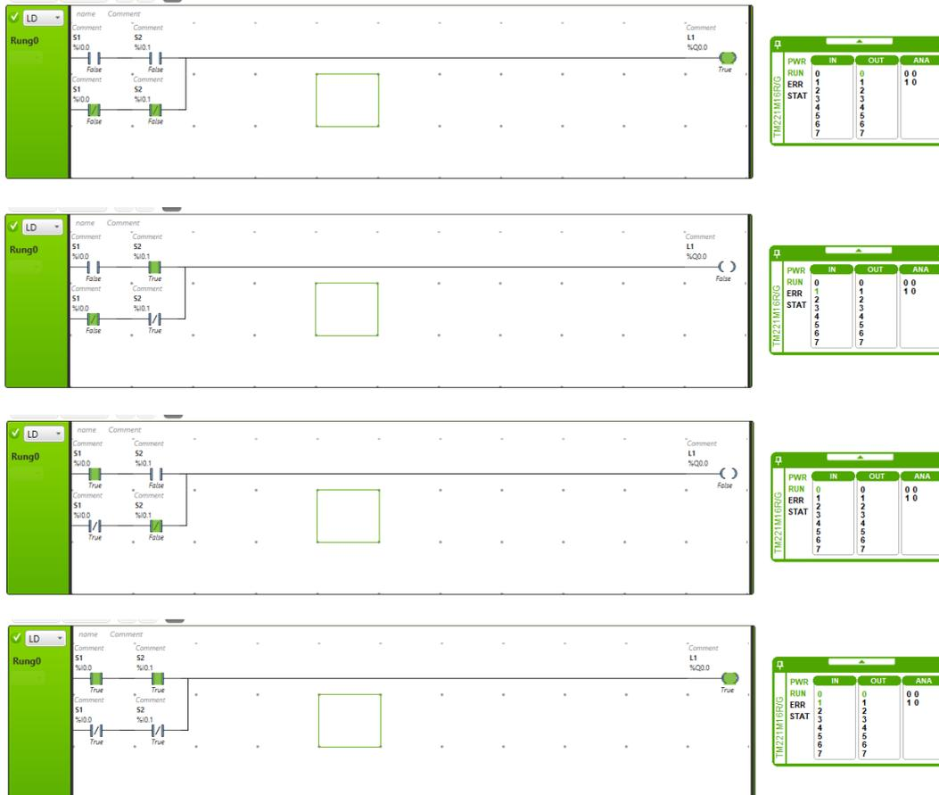
**Gambar 19.** Ladder Diagram Gerbang X-NOR
