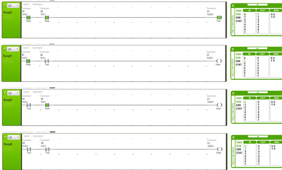
Gambar 10. Ladder Diagram Gerbang NOR
