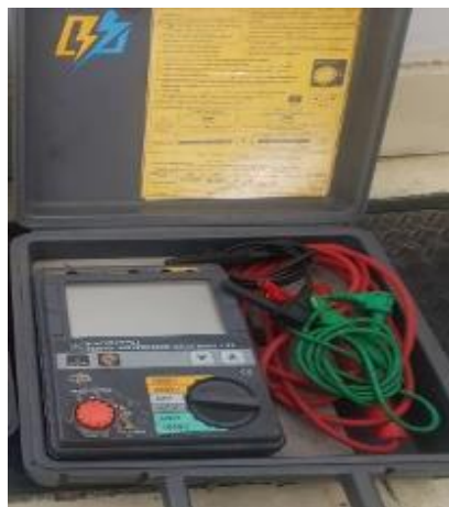
Gambar 5. Insulation Tester model 3125 merek Kyoritsu
