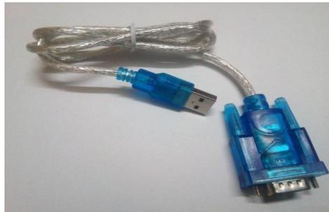
**Gambar 3.** Kabel USB to SERIAL Db 9
