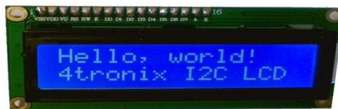
**Gambar 6 LCD 16 x 2**
