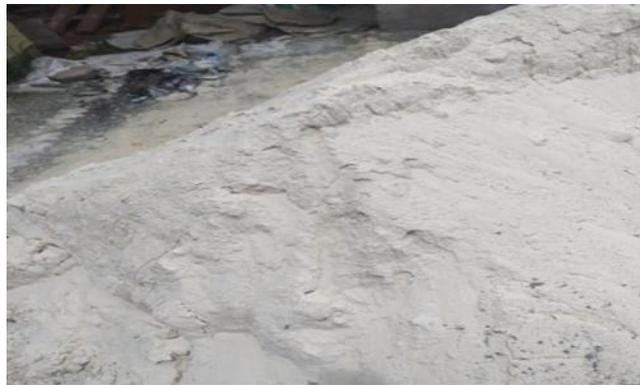
**Gambar 2. Agregat halus pasir pantai Fakfak**
